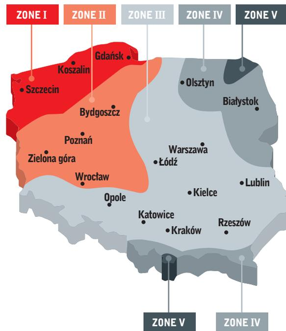
**Fig. 1.2.** Map of Poland – climatic zones for the use of bitumen 20/30 in high-stiffness modulus asphalt mixtures AC EME – zones I and II only [6]
