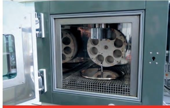
**Fig. 2.39.** General view of the oven for short-term ageing by RTFOT method (photo by ORLEN Asphalt sp. z o.o., with permission of ORLEN Laboratorium S.A.)
