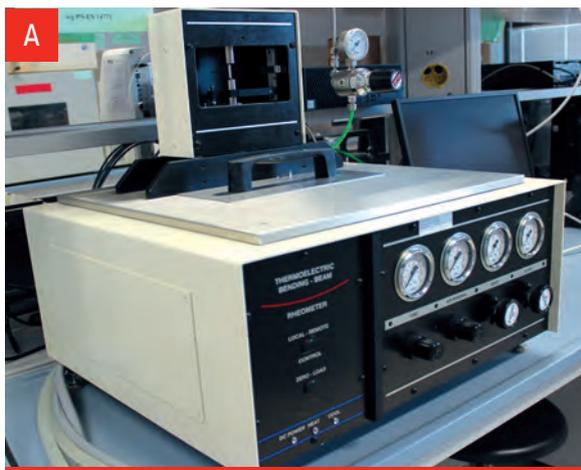
The low-temperature behaviour of the bitumen was tested using a Bending Beam Rheometer (BBR) – Fig. 3.3. The tests were performed in accordance with EN 14771:2012 and AASHTO T 313.
