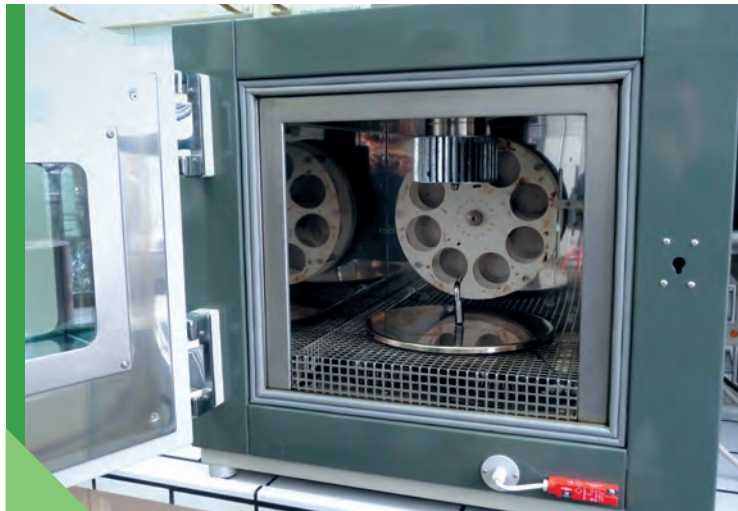
Fig. 1.39. Overview of an oven for simulation of short-term ageing using the RTFOT method (photo: ORLEN Asphalt sp. z o.o., courtesy of ORLEN Laboratorium S.A.)
