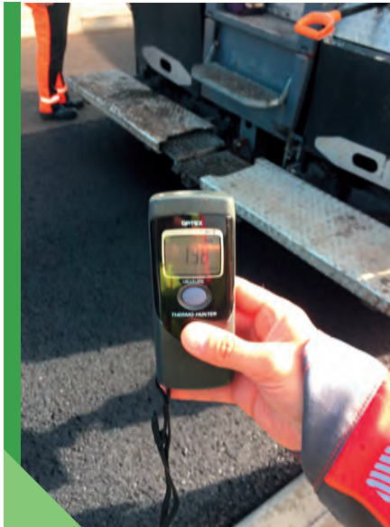
Fig.3.7. Experimental road section with bitumen 35/50 WMA constructed in 2021; measurement of the binder course temperature behind a spreader [photo K. Niemyjski, ORLEN S.A.]
