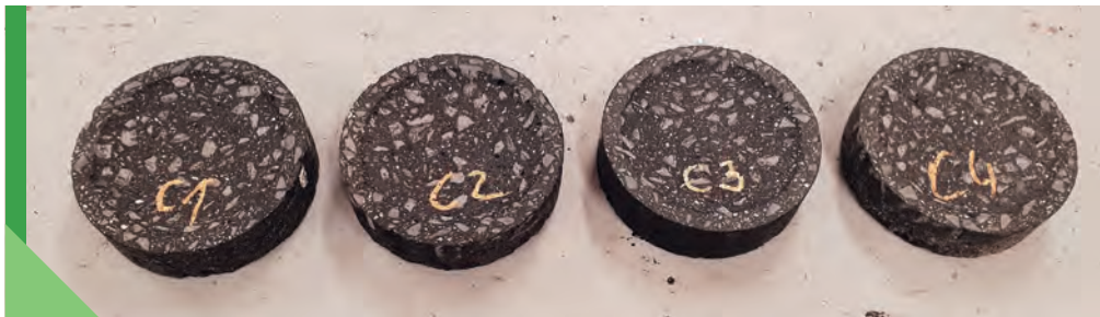
Fig. 6.3. Samples tested with the Prall method (photo P. Witkiewicz, SKANSKA AB)
