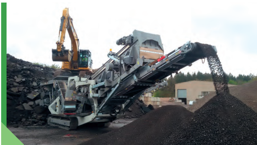
Fig. 4.3. Site-won asphalt granulator [photo Rafał Zajac, AMMANN]
