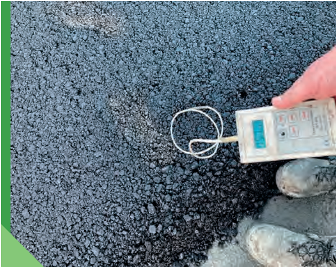
Fig. 3.16. Construction of an experimental road section using the ORBITON 45/80-80 HiMA WMA bitumen in 2021 – compacted course temperature [photo ORLEN Asfalt sp. z o.o.]
