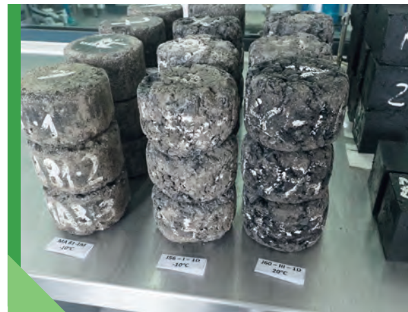
Fig. 6.7. Samples of various mixes tested with the Cantabro method (photo K. Błażejowski, ORLEN Asphalt)
