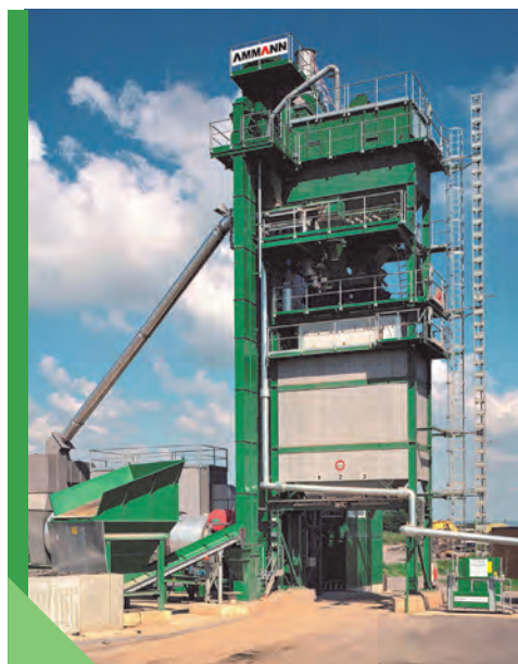
Fig. 4.5. Asphalt mix plant with not preheated RA batching system (photo AMMANN)
