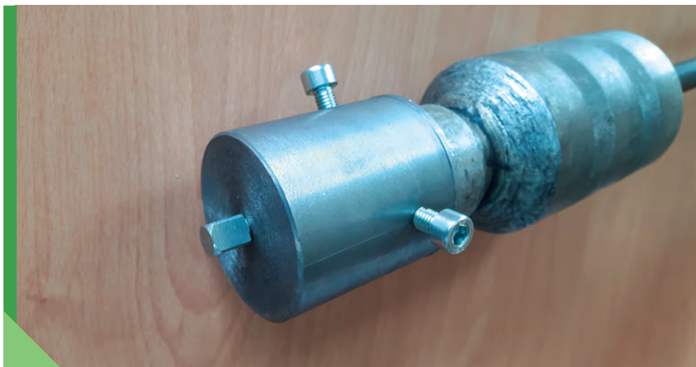
Fig. 6.4. Proctor compactor with a horseshoe nail attached (photo P. Ostrowski, ORLEN Asphalt)
