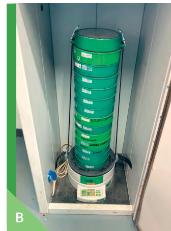
Fig. 4.4. (a) Softening point testing, R&B method (photo ORLEN Asphalt sp. z o.o., courtesy of ORLEN Laboratorium S.A.); (b) set of sieves used to determine the grain size of a mineral mix obtained from RA (photo P. Ostrowski, courtesy of Laboratorium Drogowe Wojciech Bogacki)
