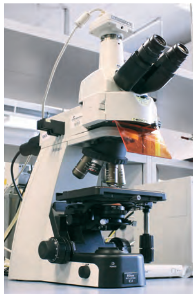
Fig. 12.4. Fluorescent microscope with UV lamp for the testing of bitumen microstructure (photo by ORLEN Asphalt Sp. z o.o., with the permission of ORLEN Laboratorium Sp. z o.o.)
