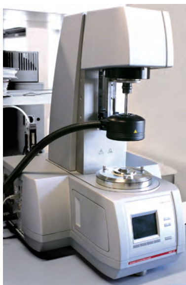
Fig. 7.1. DSR rheometer for MSCR tests (photo by ORLEN Asphalt, with the permission of ORLEN Laboratorium Sp. z o.o.)
